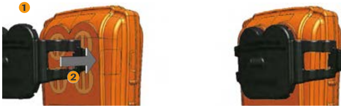
Figure 5: Fitting the calibration/bump test plate
