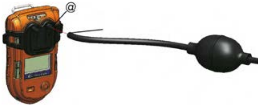
Figure 10: Attaching the Hand Aspirator
