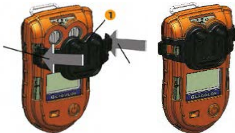
Figure 9: Attaching the Aspirator Plate
