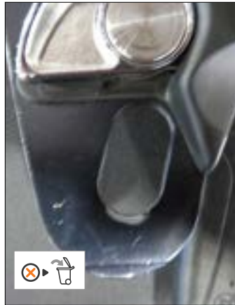
• Attachment hole deformed by a shock load
