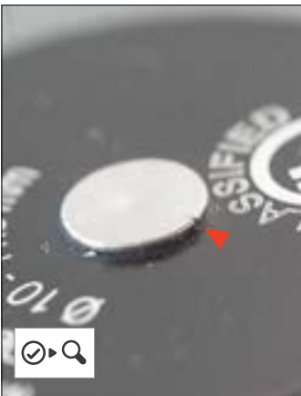
• Rivet slightly cracked
