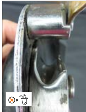
• Cam groove worn to wear indicator
