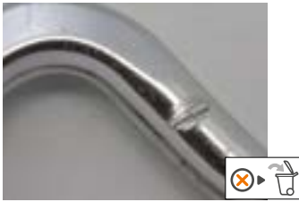
• Mark on the frame
